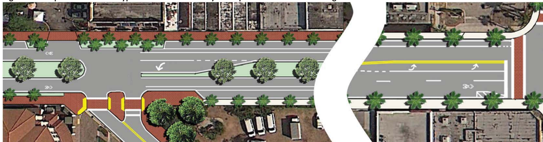
Figure 10: Proposed Road Diet Typical Sections in Vicinity of Tarpon Drive and at West Leg of SE 15 th Avenue
