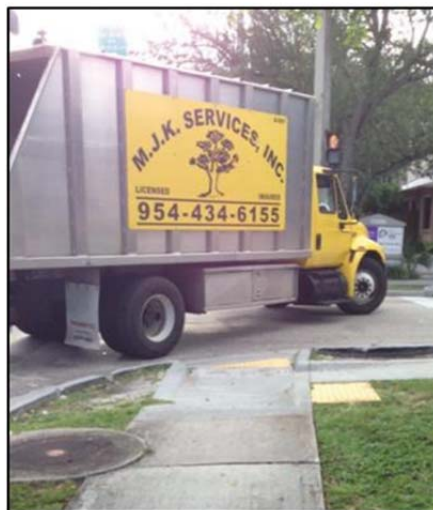
Single-unit truck turning wide at Broward Blvd; damage to curb and sidewalk
