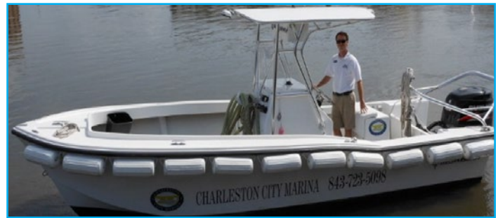
Marine Boat Builders Co. 23' 460-gallon capacity pumpout vessel used in Charleston, South Carolina
