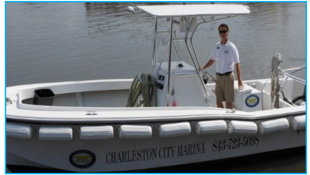
Marine Boat Builders Co. 23' 460-gallon capacity pumpout vessel used in Charleston, South Carolina
