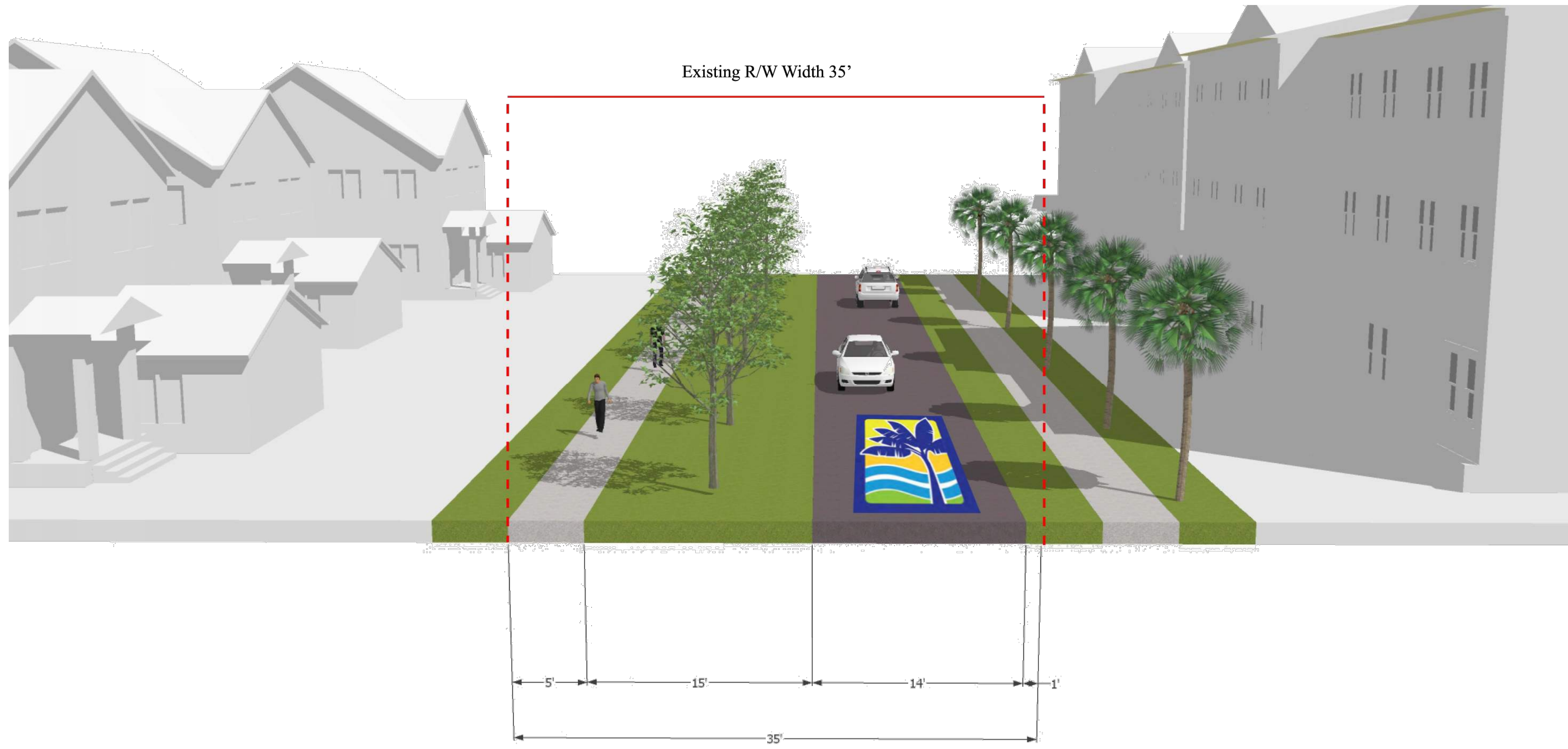
TYPICAL SECTION #3 SEGMENT 2 - ALONG NW 13TH TERRACE GOING NORTH TO SOUTH STA. 16+50 TO STA. 20+50
