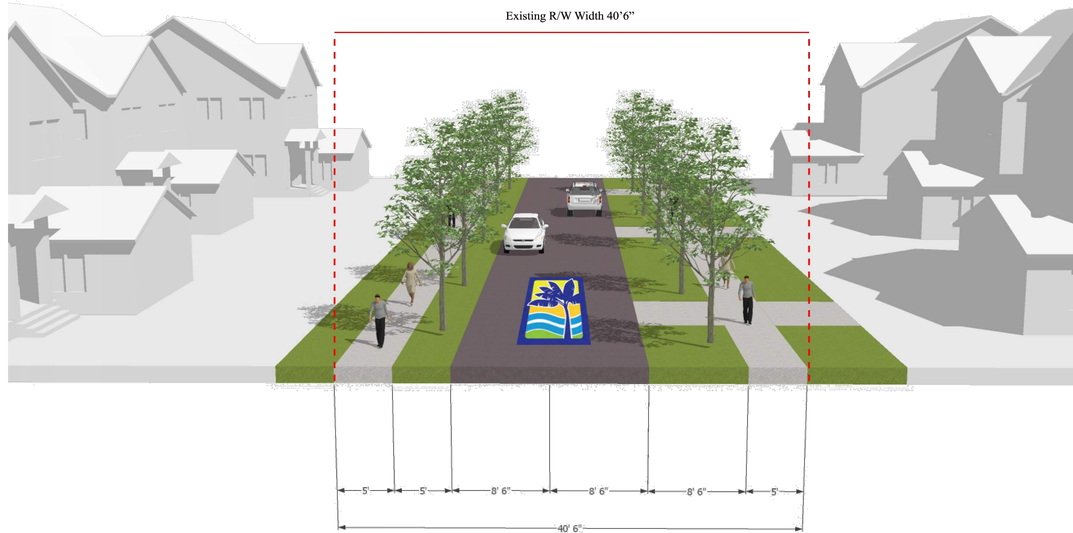
TYPICAL SECTION #7 SEGMENT 2 - ALONG NW 12TH AVE GOING NORTH TO SOUTH STA. 34+00 TO STA. 38+50
